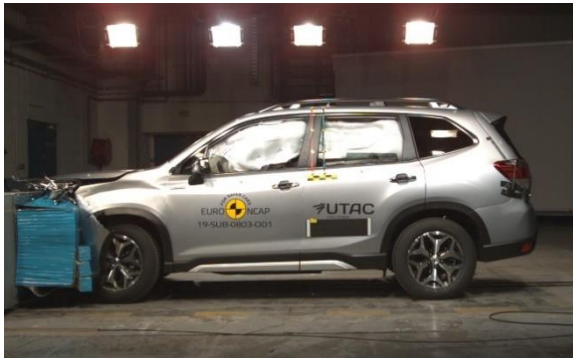
Euro NCAP impact test on Subaru Forester e-BOXER (European specs.)
