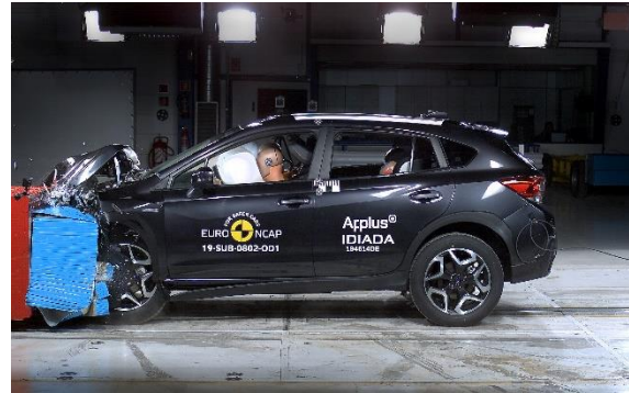
Euro NCAP impact test on Subaru XV e-BOXER (European specs.)
