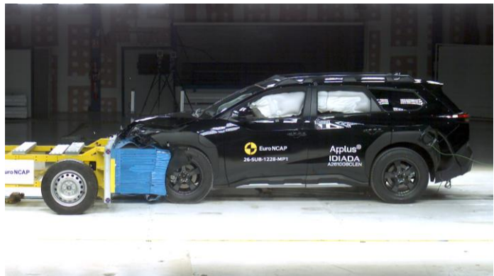
Euro NCAP impact test on E-Outback
