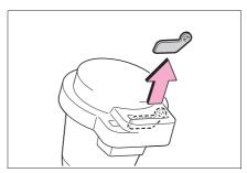
3 Remove the plug-cord connector cap.
