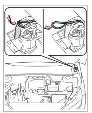
3 After unlocking the AC charging connector, fix the handle of the emergency release wire to the attachment.
