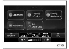
Touch (X-MODE), (Vehicle Control), (More Settings) or (A) (Auto Start Stop) to display the items that are changeable while driving.
