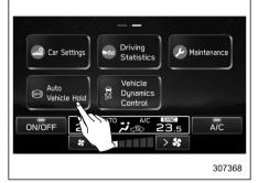
To turn the Auto Vehicle Hold function on and off. touch the "Auto Vehicle Hold" icon. When the Auto Vehicle Hold function is turned off, the Auto Vehicle Hold indicator light will turn off.
