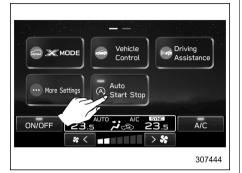
Touching "Auto Start Stop" deactivates the Auto Start Stop system and turns off the Auto Start Stop indicator (green) on the screen. Touching "Auto Start Stop" again activates the Auto Start Stop system and turns on the Auto Start Stop indicator (green).
