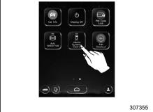
To turn the Vehicle Dynamics Control on and off, touch the "Vehicle Dynamics Control" icon.
