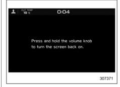
2. Press and hold the volume knob to turn the screen back on.
