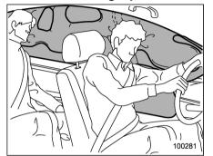
The driver's and front passenger's SRS side airbags and SRS curtain airbags deploy independently of each other since each has its own impact sensor. Therefore, they may not both deploy in the same accident. Also, the SRS side airbag and SRS curtain airbag deploy independently of the driver's and front passenger's SRS frontal airbags in the steering wheel and instrument panel.
