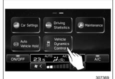
To turn the Vehicle Dynamics Control on and off, touch the "Vehicle Dynamics Control" icon
