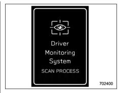
1. When the door is opened and the push-button ignition switch is OFF, the user recognition screen appears and the Driver Monitoring system starts user recognition.
