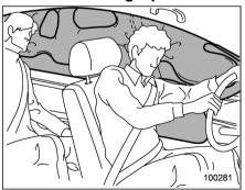
The driver's and front passenger's SRS side airbags and SRS curtain airbags deploy independently of each other since each has its own impact sensor. Therefore, they may not both deploy in the same accident. Also, the SRS side airbag and SRS curtain airbag deploy independently of the driver's and front passenger's SRS frontal airbags in the steering wheel and instrument panel.
