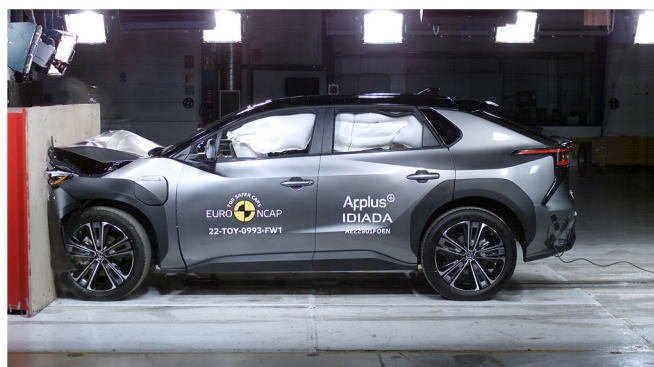
Euro NCAP impact test on Toyota bZ4X
